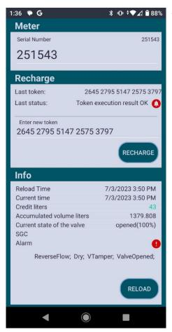
ADDRA Prepay View application allows user to send token, view valve state and meter information including meter alarms. The application has a simple and clear interface.
