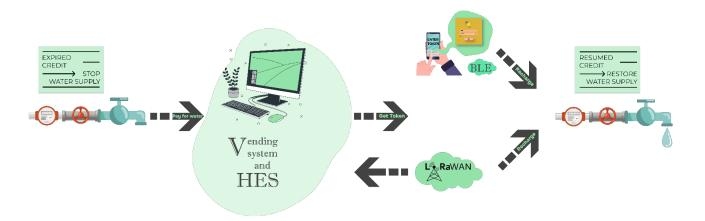
A customer is required to pay for water and send the received token for replenishment of the credit to the meter locally by a special mobile application or remotely from HES via LoRaWAN.
